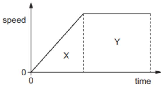
Which area represents the distance travelled while the car is accelerating?
